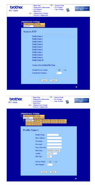
Enter the name that you want to use for the profile of the FTP server. This name will be displayed on the LCD of the machine and can be up to 15 characters.
