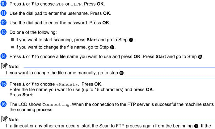
If a timeout or any other error occurs, start the Scan to FTP process again from the beginning ①. If the user name is entered incorrectly then the LCD will show Authenticate Err, please start the process again from the beginning ①.
